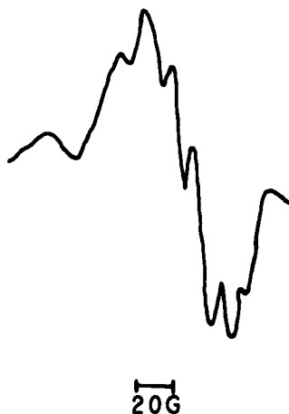
FIG. 2. ESR spectrum of radicals formed by treatment of a glass tube with N_2 plasma at a pressure of 12 mTorr N_2 , 30 W power for 5 min with subsequent exposure of the tube to air.
